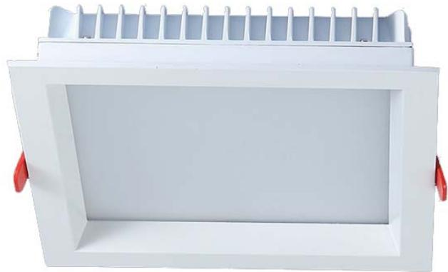
The Atlas Orion Deep Max is a 180 x 180mm low void downlight which uses a Samsung LED engine. The Orion Deep Max has a 10mm recessed bezel feature for anti-glare cutoff. The heatsink is constructed from die-cast aluminium complete with aluminium bezel and reflector. The heatsink features spring arms which allows the downlight to be installed with ease.
