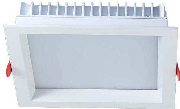
The Orion Deep is a 140 x 140mm low void downlight which uses a Samsung LED engine. The Orion Deep has a 10mm recessed bezel feature for anti-glare cutoff. The heatsink is constructed from die-cast aluminium complete with aluminium bezel and reflector. The heatsink features spring arms which allows the downlight to be installed with ease.
