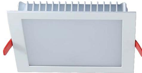
The Orion Mini is a 104 x 104mm low void downlight which uses a Samsung LED engine. The heatsink is constructed from die-cast aluminium complete with aluminium bezel and reflector. The heatsink features spring arms which allows the downlight to be installed with ease.
